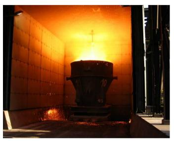
PROBLEM: CaO → not volume stable → bound the CaO by SiO2 → Generate oxydation heat by adding O2
